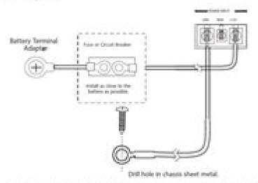
Make the ground lead as short as possible, leaving enough length to complete the installation. To ensure a good ground, scrape away any paint or undercoating to expose bare metal. Use a "ring" terminal of the proper gauge and an "outside star washer" (between the chassis and ring terminal) when making your ground connection.
