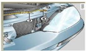
Lift the bonnet, release stay 4 from its holder 3 and, for your own safety, it is very important to fix it into retainer 5 in the bonnet.
