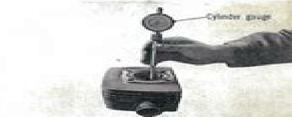
Fig. 6-2-1 Measuring cylinder bore
