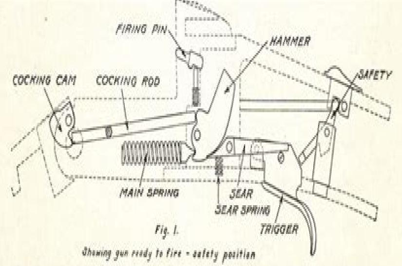
Lock Mechanism of Lefever Doubles Coil Springs—no flat springs to break or render LEFEVER ARMS COMPANY, Incorporated, Ithaca, N. Y.
