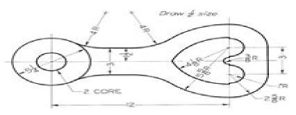
Fig. 5-37. Locomotive Truck Swing Link.\*
