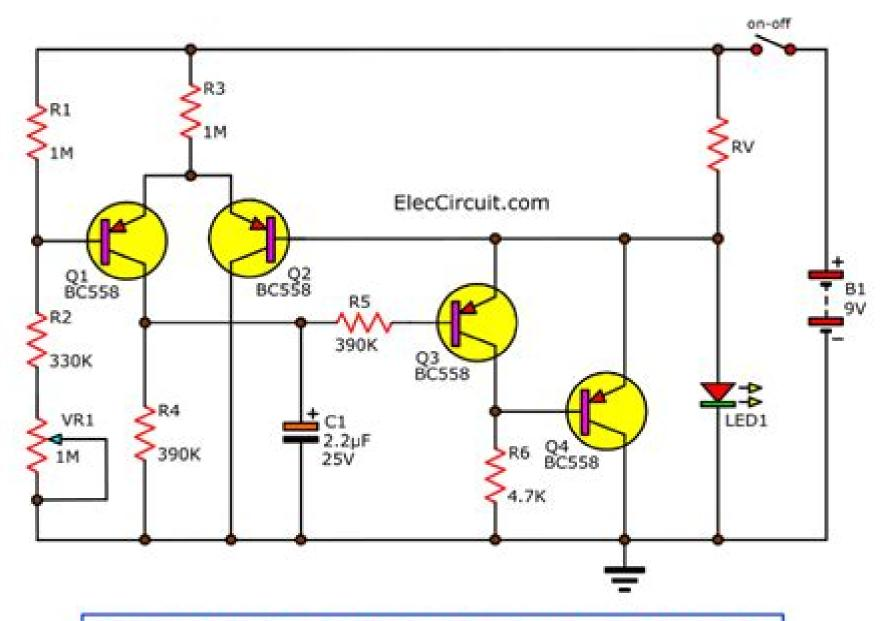
LED battery status indicator circuit using 4 Transistors
