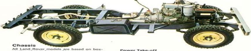
All Land-Rover models are based on boxsection chassis frames of immense strength, built to withstand the constant shocks of day-in, day-out, cross-country operation. They are painted inside as well as outside and are therefore resistant to rust and corrosion over very long periods of use.
