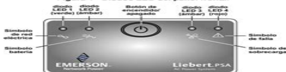
Figura 1 - Diodos LED del panel frontal
