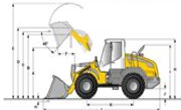
Fig. 4: Complete machine with loading bucket (Z kinematics)
