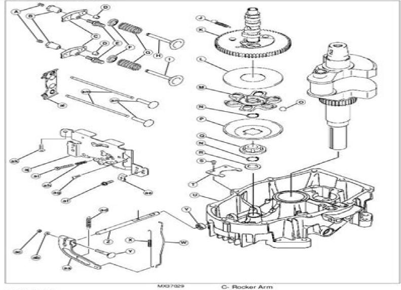
A- Lock Screw B- Rocker Nut C- Rocker Arm D- Spring Collet
