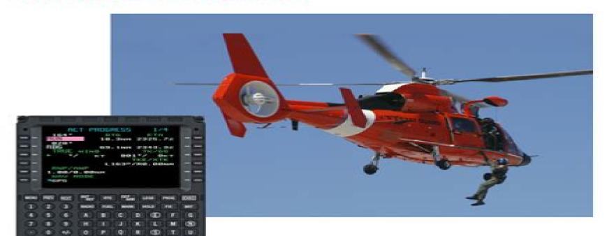
The CMA-9000 is an industry leading Flight and Radio Management System (FMS/RMS) designed for demanding commercial, paramilitary and military helicopter applications.
