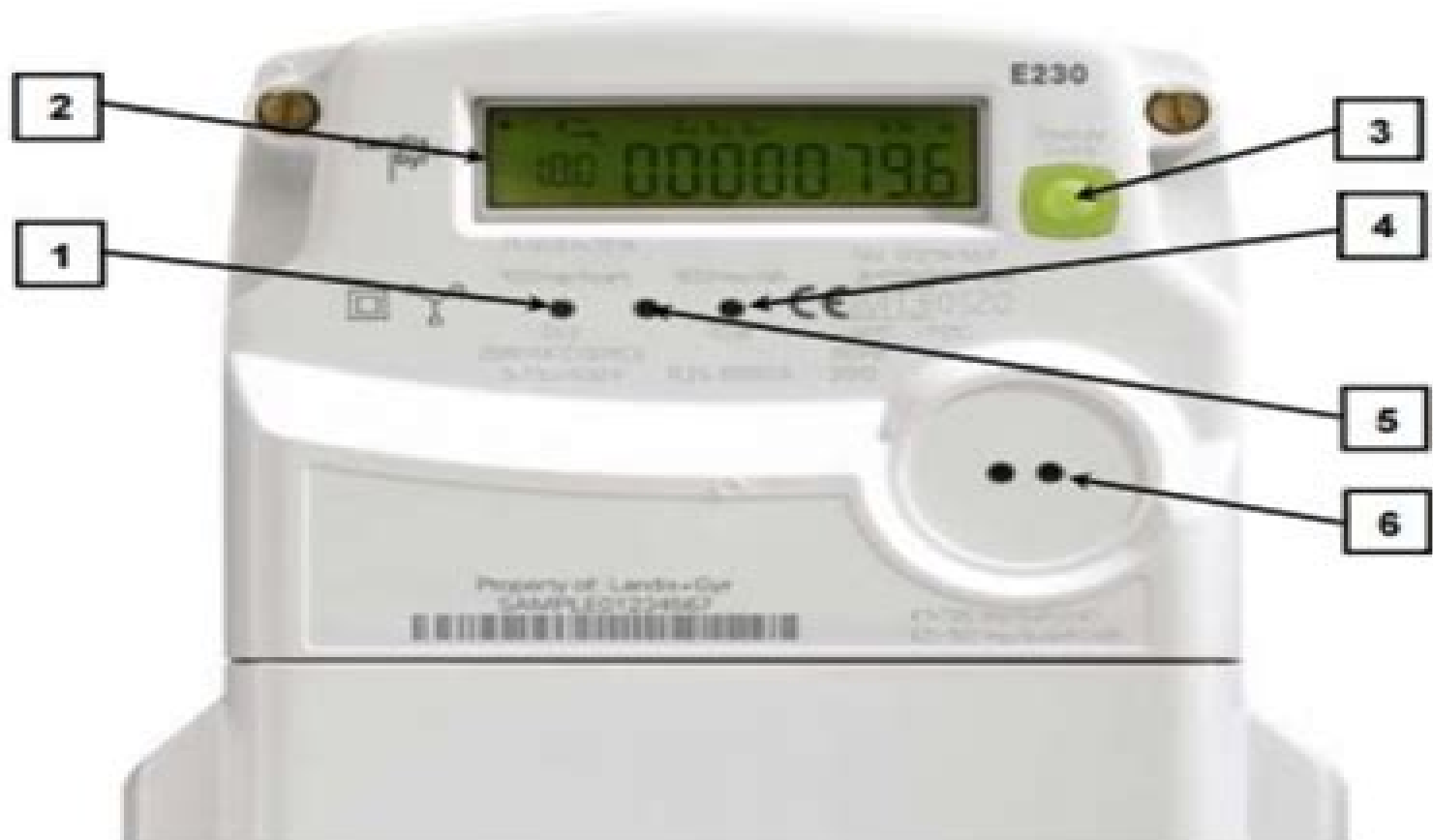
Figure 3. View of the E230 ZxR110CC meter
