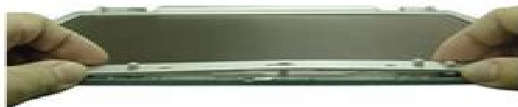
Fig. 28 Removing the LCD front cover
