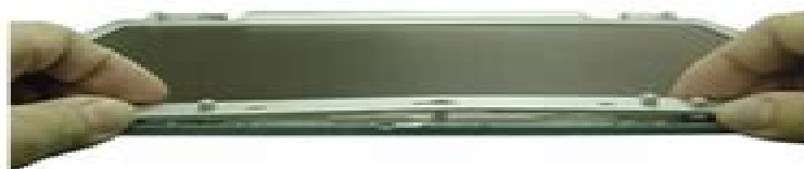
Fig. 28 Removing the LCD front cover
