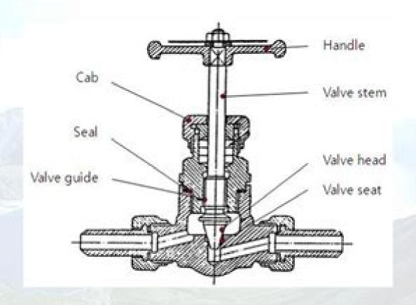
Fig. Manual type expansion valve (cone type)
