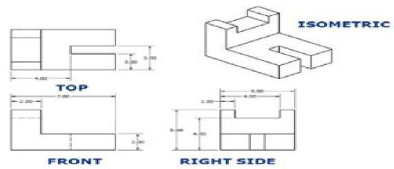
Each is an orthographic projection of a particular aspect of a threedimensional object or construction.
