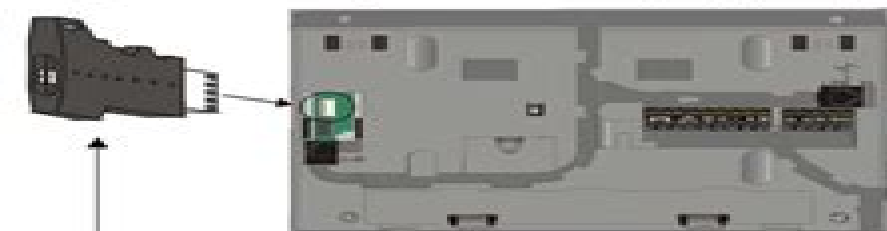
Figure 13: Connecting a Paradox Memory Key (PMC-3)
