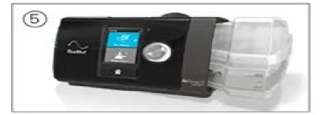
Close the water tub and insert it into the side of the device.
