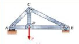
A truss consists of straight members connected at joints. No member is continuous through a joint.
