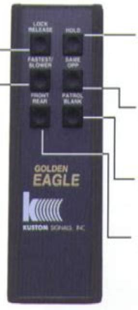
Hold controls the transmission of RF signal, defeating radar detectors.
