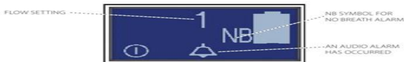
Figure 18. Example of an alarm screen. If the device does not detect breathing for 120 seconds, it will sound the NB alarm and show this typical display with the NB alarm symbol (NB = No Breath). The alarm symbol (bell) shows the audio alarm is on. To silence the audio alarm, press the alarm symbol. For a complete list of alarms, see the Alarm Indicators section of this manual.
