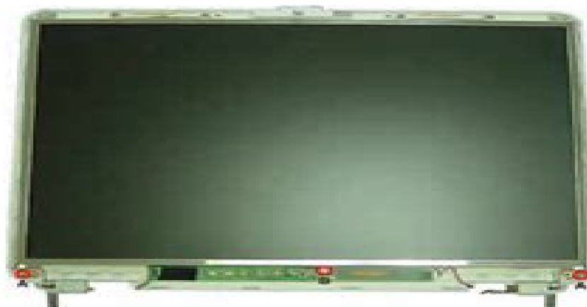
Fig. 29 Removing the LCD panel screws
