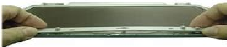
Fig. 28 Removing the LCD front cover
