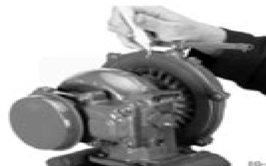
Figure 2.10 Mark Compressor/Backplate Location
