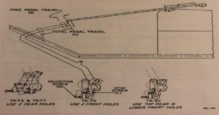
The three inset illustrations show the mounting of the clutch release cam for the different transmissions used in "B" model vehicles.
