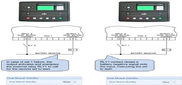
Screen capture from DSE Configuration Suite PC Software showing the configuration of the Master and Slave controllers.
