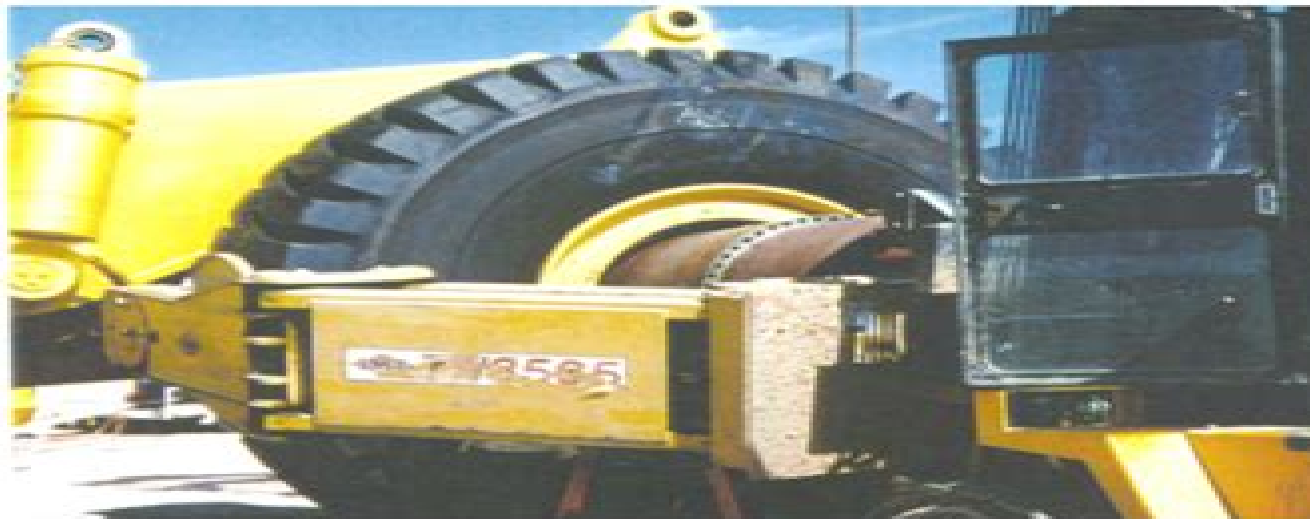
FIGURE 6-89. INNER REAR TIRE INSTALLATION WITH TIRE HANDLER
