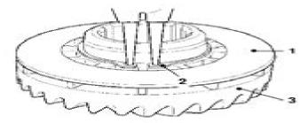
Install the oil deflector (1) and the locking ring (2) on the gear wheel (3).
