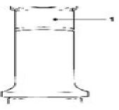
Press on the bearing race (1) on the propeller shaft (in case it has been dismantled).
