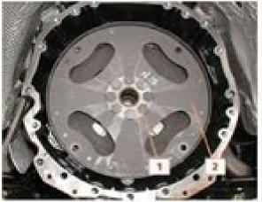
Undo all the fastering screws (1) and remove the complete engine flywheel (Flexplate) (2).
