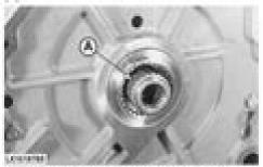
Remove needle bearing (A) with thrust washers.
