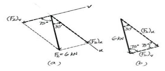
Ans:  $(F_2)_v = 6.00 \text{ kN}$  $(F_2)_v = 3.11 \text{ kN}$
