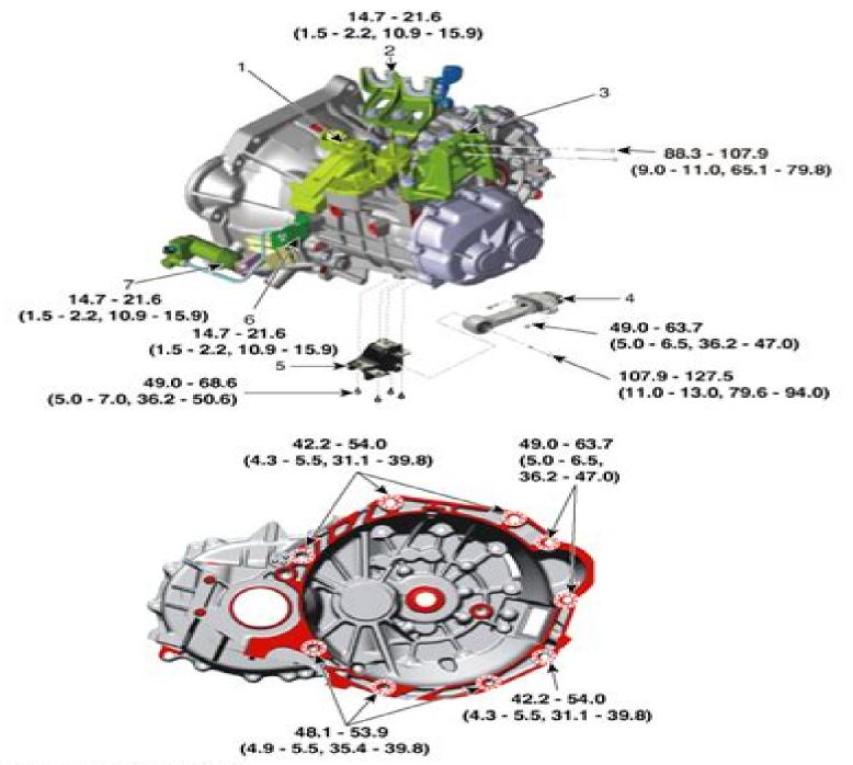
Tightening torque: N-m (kgf-m, lb-ft)
