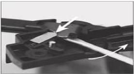
Press down the hand guard in the correct position.
