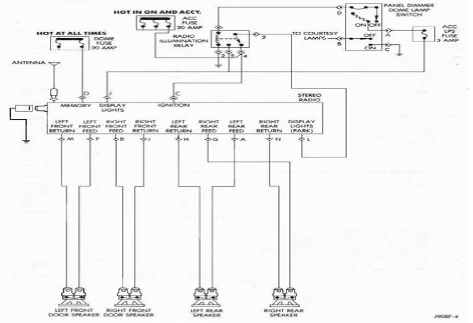
Fig. 3 Radio Schematic - SJ
