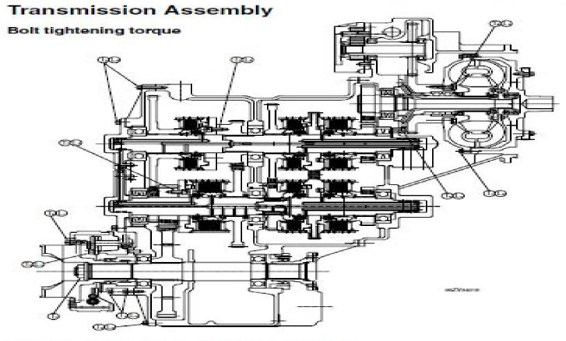
T.: 392 N-m ( 40 kgf-m) (289 lb-ft) (Molybdenum disulfide greese / MOS<sub>2</sub> application)
