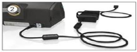
Plug the power connector into the rear of the device. Connect one end of the power cord into the power supply unit and the other end into the power outlet.
