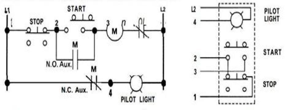
Bulletin 1495 normally closed auxiliary contacts are required. With the motor running contacts are open; with the motor stopped contacts are closed and the pilot light is illuminated. The basic circuit and its operation is the same as the diagram on Page 6.
