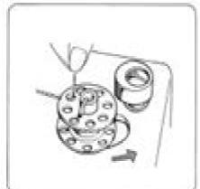
Draw thread from spool. Pass the thread through the top cover thread guide. Guide the thread around the bobbin winder thread guide, Insert the thread through the hole in the bobbin, threading from the inside to the outside. Put the bobbin on the bobbin winder spindle, and push it to the right.
