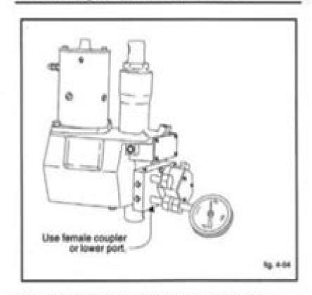
NOTE: Poor condition of the battery or motor will cause invalid test results.
