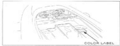
(5) The color label is attached as shown. When ordering color-coded parts, sliveys specify the designated color code.
