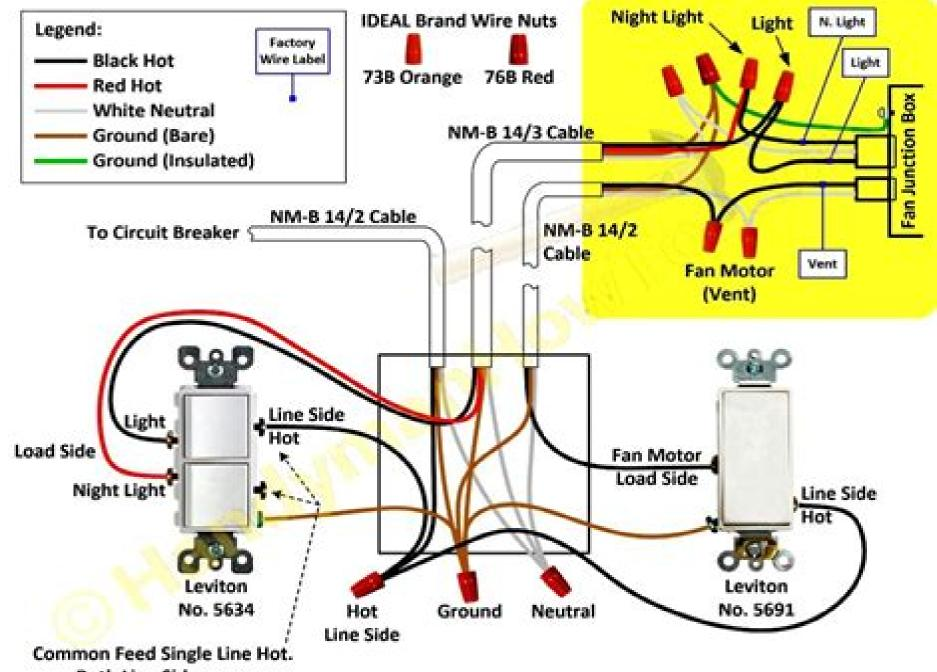
Both Line Side screws are connected by a metal Break-off fin.
