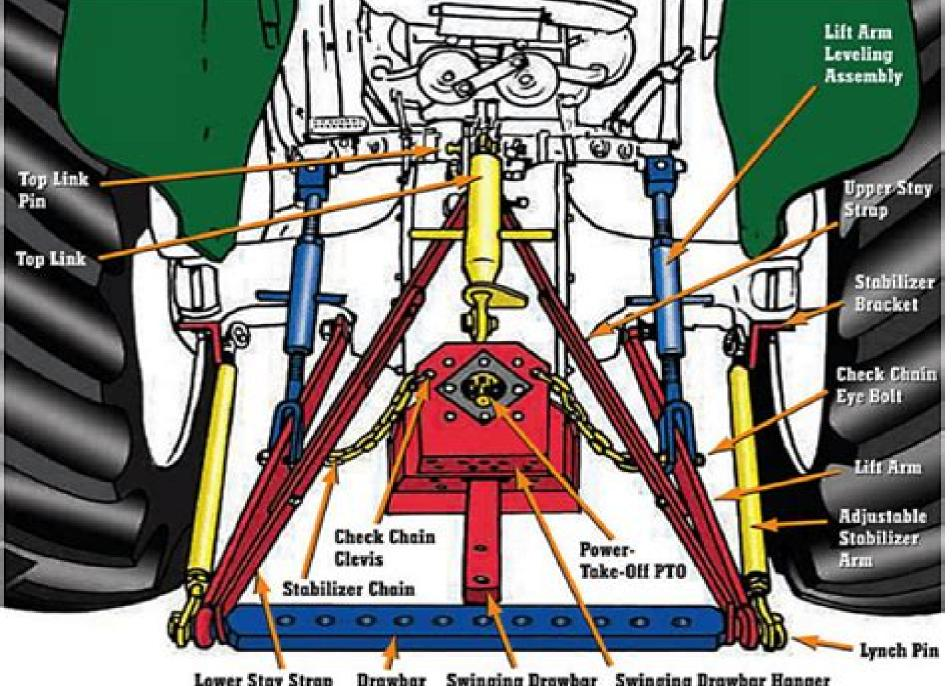
Lower Stay Strap Drawbar Swinging Drawbar Swinging Drawbar Hanger
