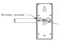
Change direction of the handle 1.Remove the criss screw in the figure, Turn the handle 180-degrees in the direction of the arrow. 2.After adjusting the handle direction, install the screw and complete the reversing.
