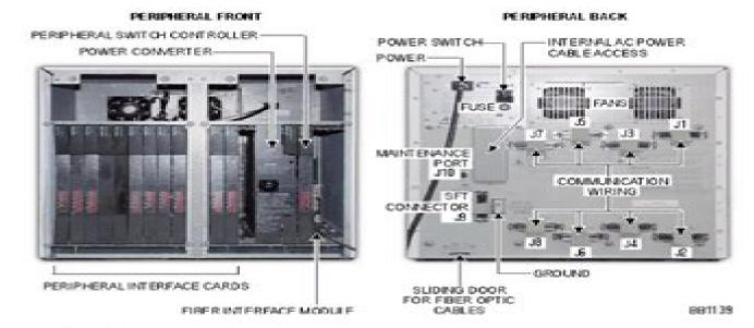
The peripheral cabinet consists of the following components:
