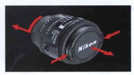
Remove body cap and front and rear lens caps.
