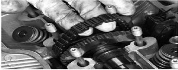
Loop the cam chain over the sprocket.
