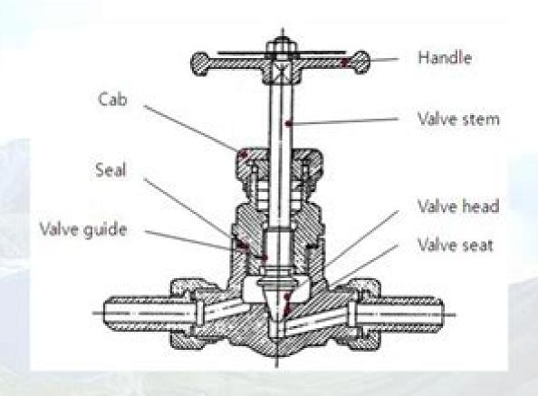
Fig. Manual type expansion valve (cone type)
