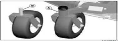
The two front caster wheel supports (A) utilize sealed bearings, which do not require lubrication. There are no grease fittings in the wheel supports.
