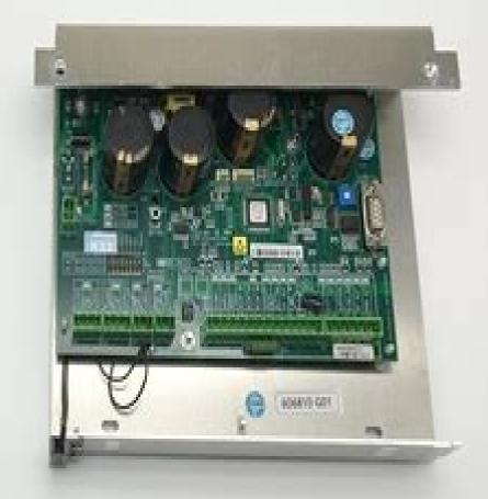
KONE Elevator AMD Door Drive Inverter (KM606800G01 / 606810G01)
