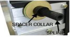
Install the Spline and the Spacer Collar. Install the Motor onto the Spline. Install the Black Bolt and Washer onto the Motor and Tighten to Approximately 70 Foot Pounds
