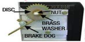
Lower the Boat Lift. Remove the Acorn Nut. and Wheel. Remove the Brake Dog, Brass Washer and the Disc. You Will Not Use Them Anymore.
