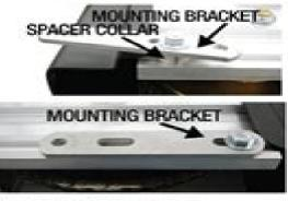
This Lift has Two Options, One for Left or Right Mounting. Install the Mounting Bracket.
