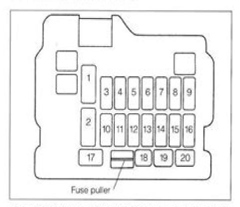
NOTE: Spare fuses are contained in the fuse housing. Always use a fuse of the same capacity for replacement.
